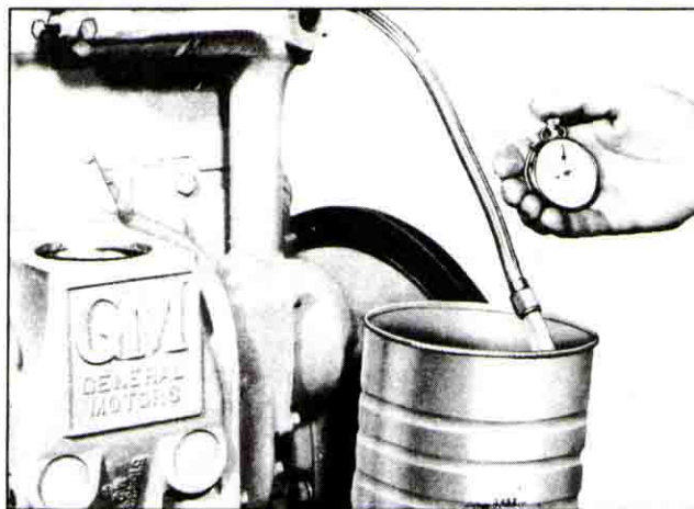
Fig. 17 - Measuring Return Fuel Flow
